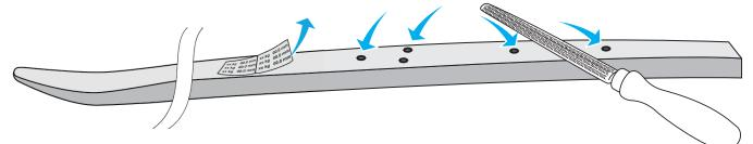
2/ CLEAN THE SKI SURFACE WITH THE PROVIDED WIPE 15CM AHEAD OF THE FRONT HOLE. USE THE WIPE ONLY FROM BACK TO FRONT
